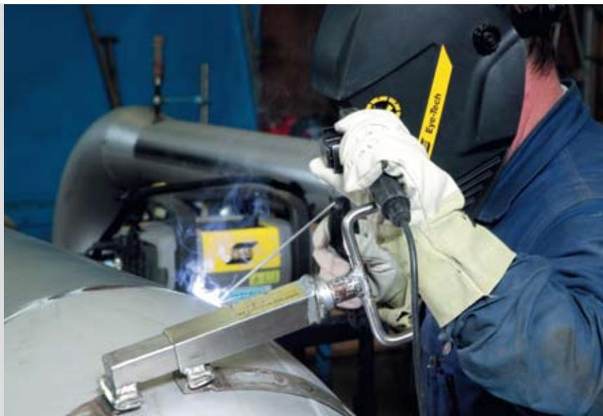
**OK 61.20 used for the vertical down welding of water supply piping in the pipeshop at a paper and pulp plant (AISI 304, 2.5 mm wall thickness). The remote control on the CaddyArc portable inverter is used to prevent burn-through by controlling the arc which is directed at the root of the joint. Welding is carried out in the two o'clock position while the pipe is rotated upwards, manually.**
