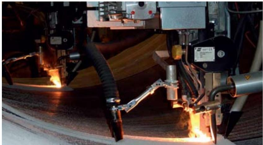
melts the surface of the base material and the strip electrode end, which is dipping in the slag and the flux. The penetration is less for ESW than for SAW since there is no arc between the strip electrode and the parent material.
